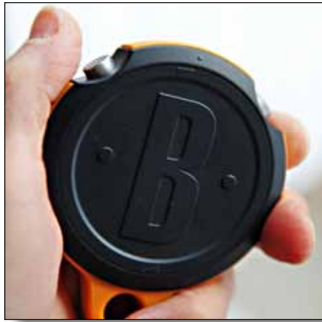
Figure 2. Battery cover on the back. Arrows indicating direction to open are small and contours low, giving poor traction. Distance between open and close is small and the end position poorly felt. After opening, the cover remains on and the unit must be turned over to have it fall off.
