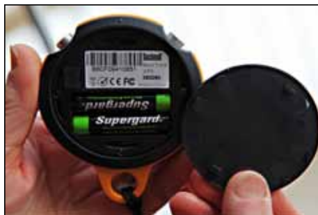
Figure 3. Once uncovered, the batteries are easy to remove and replace. Replacing the cover is more difficult and it may remain incompletely closed, allowing dirt and small particles to get inside, or potentially even losing the cover. The problem with the cover seems to be corrected in the new model.
